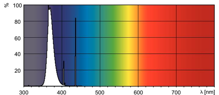
XDPB\_XUBTL\_10-Spectral power distribution B/W
